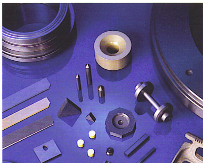
Typical parts finished by diamond wheel grinding. Photo courtesy of PremaTech Advanced Ceramics.
